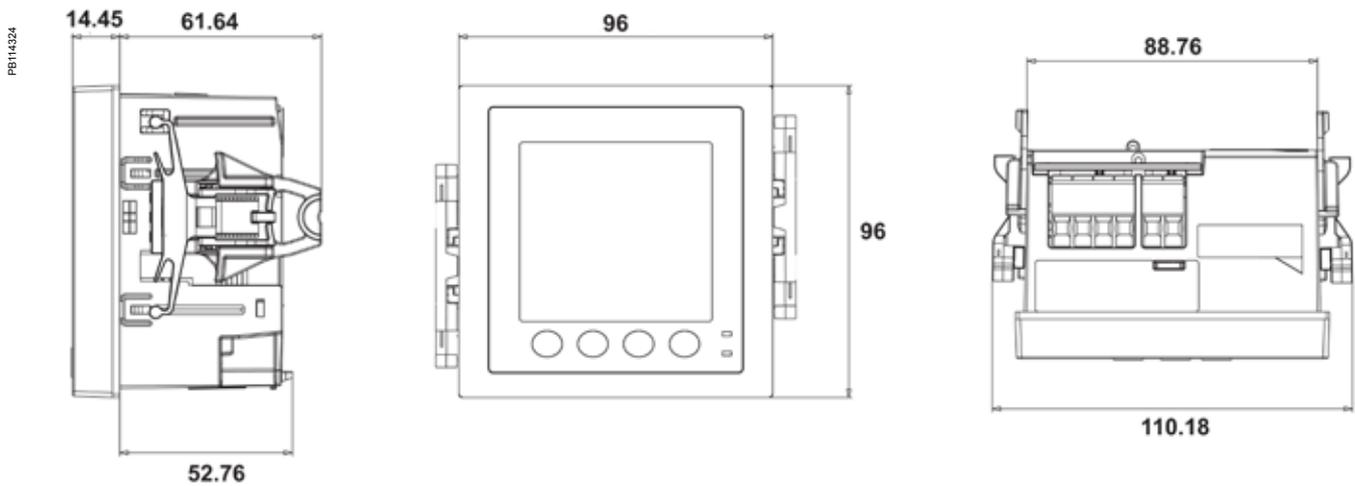
**PM2000 I/O module mechanical dimensions**
