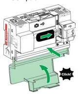
For 3G modems that do not mount inside the Com'X 200/210 front cover, break off the tab to create an opening for the cable, then connect the modem cable to the internal USB port. Com'X 200/210 User Manual Settings
