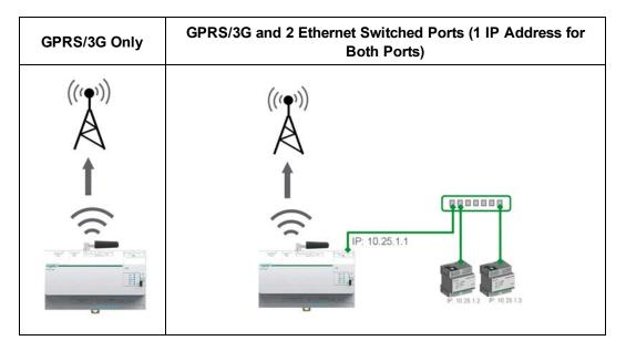
GPRS/3G access can be added to the Com'X 200/210 by installing a modem under the cover.
